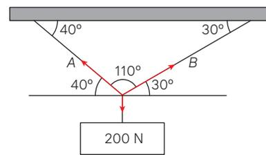
$$\frac{T_A}{\sin 120^\circ} = \frac{T_B}{\sin 130^\circ} = \frac{200}{\sin 110^\circ}$$
